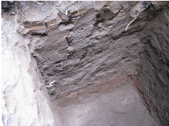
CB34 looking south. Face in the slot showing the sandy layer beneath the 'concrete' at the top. Sandy clay beneath this and the red clay at the bottom. The red clay forms a thinning layer and is not seen on the north side. It is possibly Anglian till.
