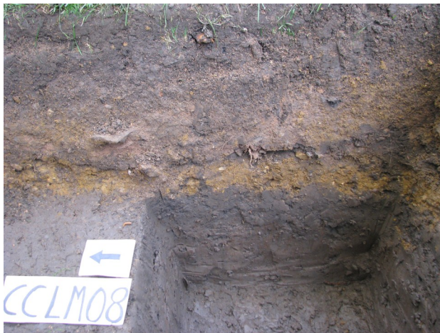
IMG_1960 East wall final depth showing sand and gravel lying on clay at about 35 cm depth. The transition downwards from the subsoil in the lake clay takes place within the slot
