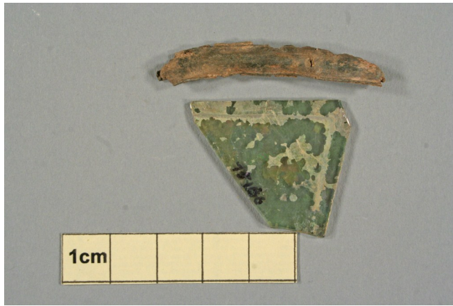
A piece of glass from a diamond shaped pane marked where it has been set in lead. Above it is a piece of window lead. The glass is 1/16th inch thick.
