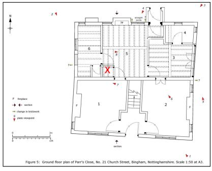
The ground floor front rooms are tall in height, are well lit by front and side windows and both rooms have fireplaces set in the end walls. There is only one staircase, a straight flight that rises from immediately behind the front door to an enclosed landing in the upper part of rear range (see below right). Before about 1990 the main
